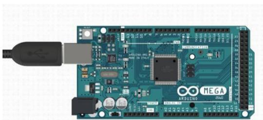
Fig-3: Arduino Mega
